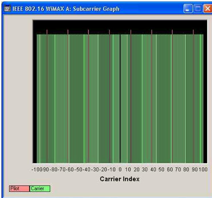
The graph shows used pilots and carriers of the current subchannelization mode. When subchannelization is activated by setting **No. of used Subchannels** to a value different than 16, the graph shows the used and blanked carriers according to the setting of **Subchannel Index**.
